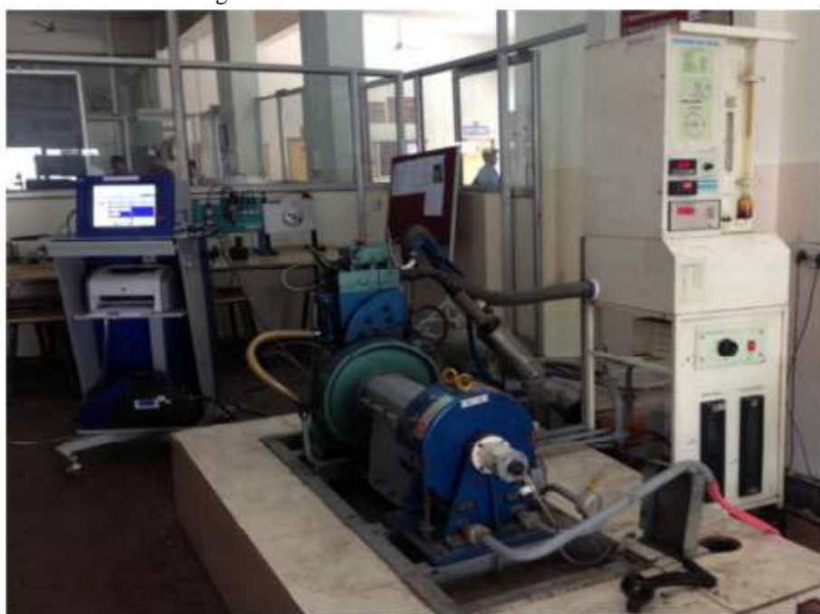
Figure 1 Experimental Setup with engine and analyzer
