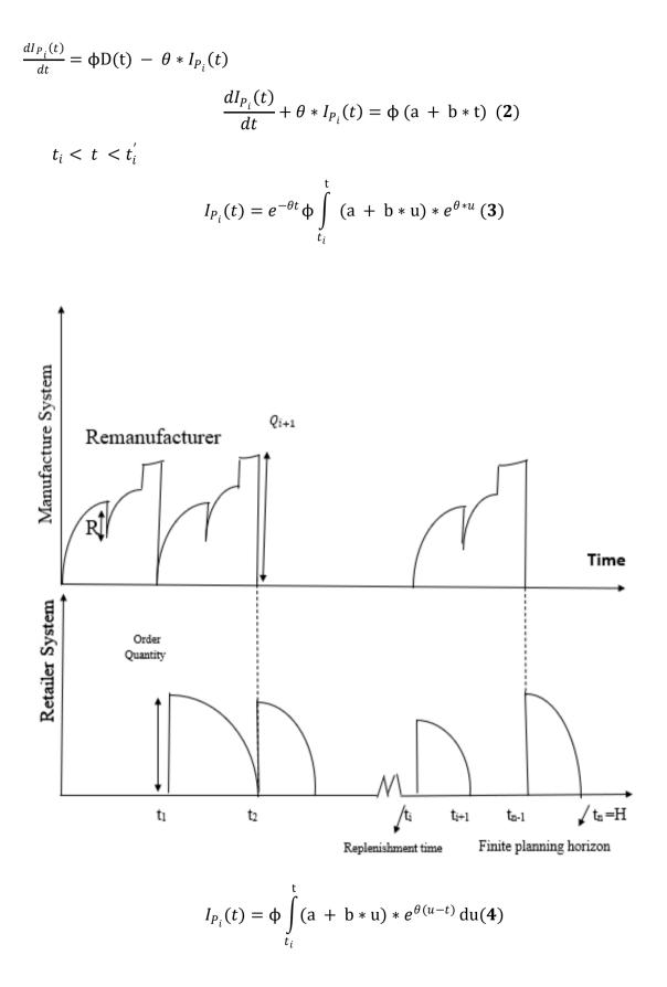
Figure 1 Production level of supplier and Replenishment to retailers.
