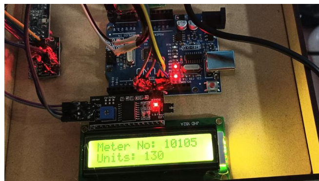
Fig.17: Showing LCD that Meter Number and No. of units used in receiver section
