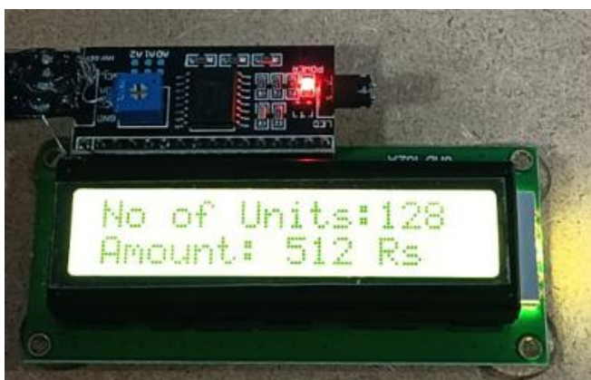
Fig.14: Showing LCD that No. of units used and amount for used units in transmitter section
