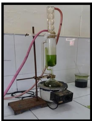
Fig 2. Extraction process through Soxhlet apparatus.
