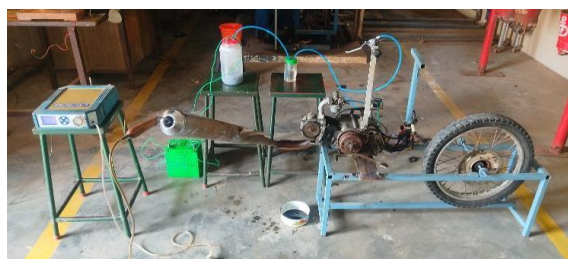
Fig. 3. Experimental Setup with Gas Analyzer
