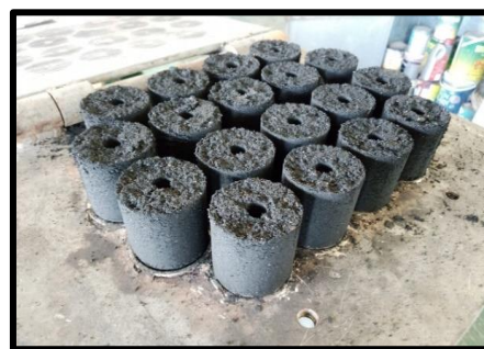
Figure 6. The developed charcoal briquettes from vegetable and fruit wastes
