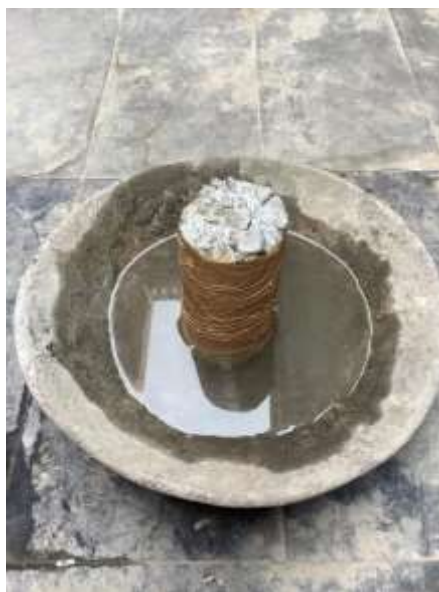
Figure 2.5 Water Absorption test on GPA concrete
