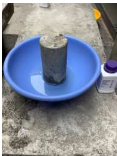
Figure 2.8 GPA concrete immersed in sodium sulfate solution
