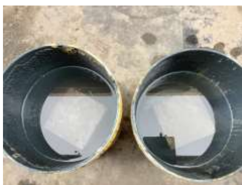
Figure 2.7 GPA concrete specimen immersed in H 2 SO 4 and Hcl acids
