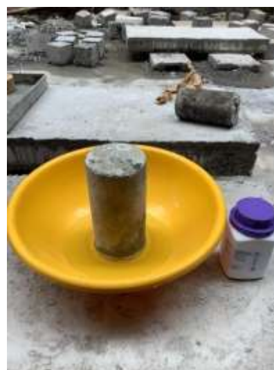
Figure 2.9 GPA concrete immersed in sodium chloride solution
