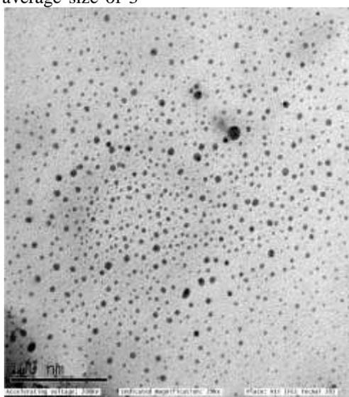
Fig.3. Transmission Electron Microscopic image of silver nanoparticles synthesized by bromelain extracts.
