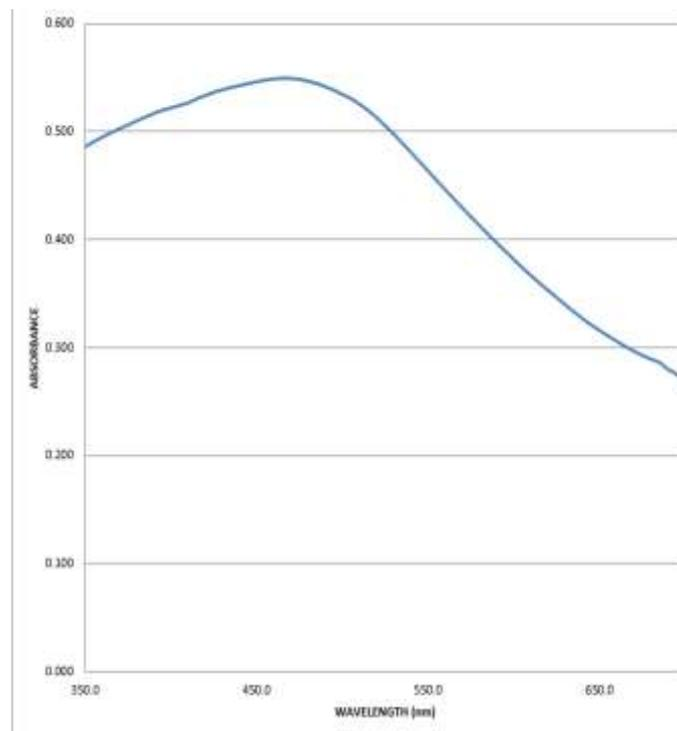
Fig.2. UV-vis spectra of silver nanoparticles synthesized by bromelain extract show the SPR band at 460nm confirming the formation of silver nanoparticles in the reaction mixture.
