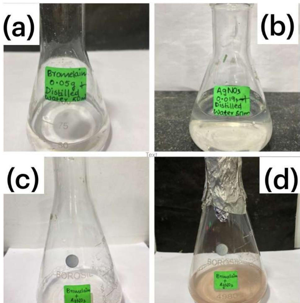
Fig.1. Visual observation showing (a) formulation of bromelain extract, (b) formulation of silver nitrate solution,(c) reaction mixture of bromelain extract and silver nitrate (d) colour change of reaction mixture after 24h.
