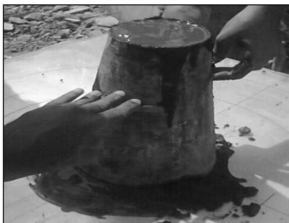
a. Concreting the Slump Cone
