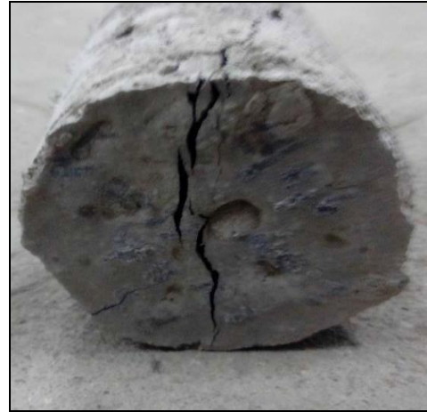
b. Cylinder after Testing
