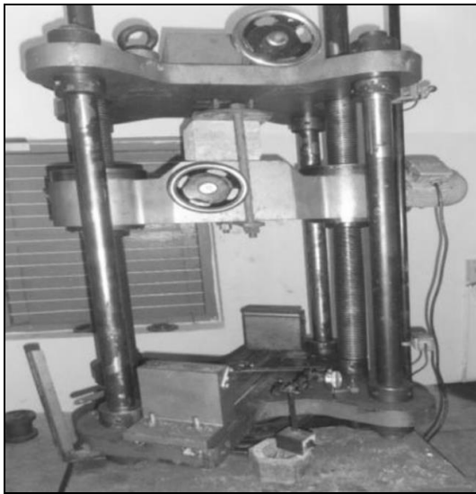
a. Cube embedded with steel rod under Loading
