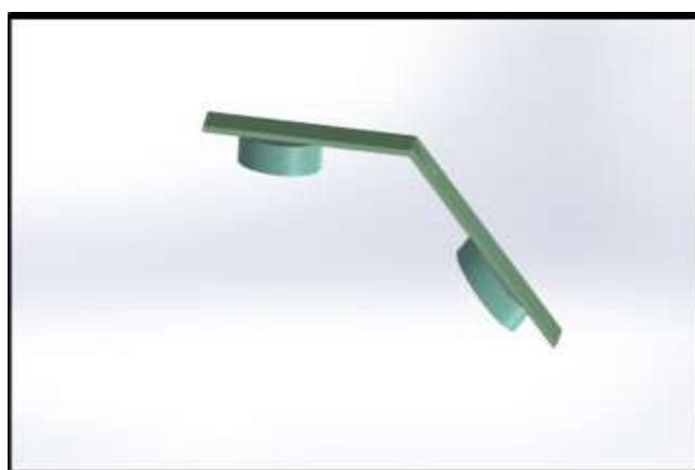
Figure 2. Electromagnetic Gripper
