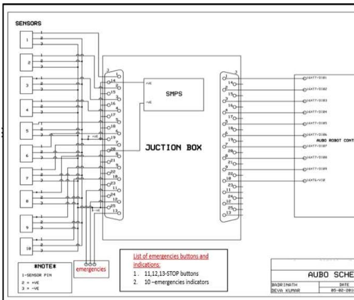
Figure.4 Overall Schematic of pick and place operation in clutch diaphragm spring testing
