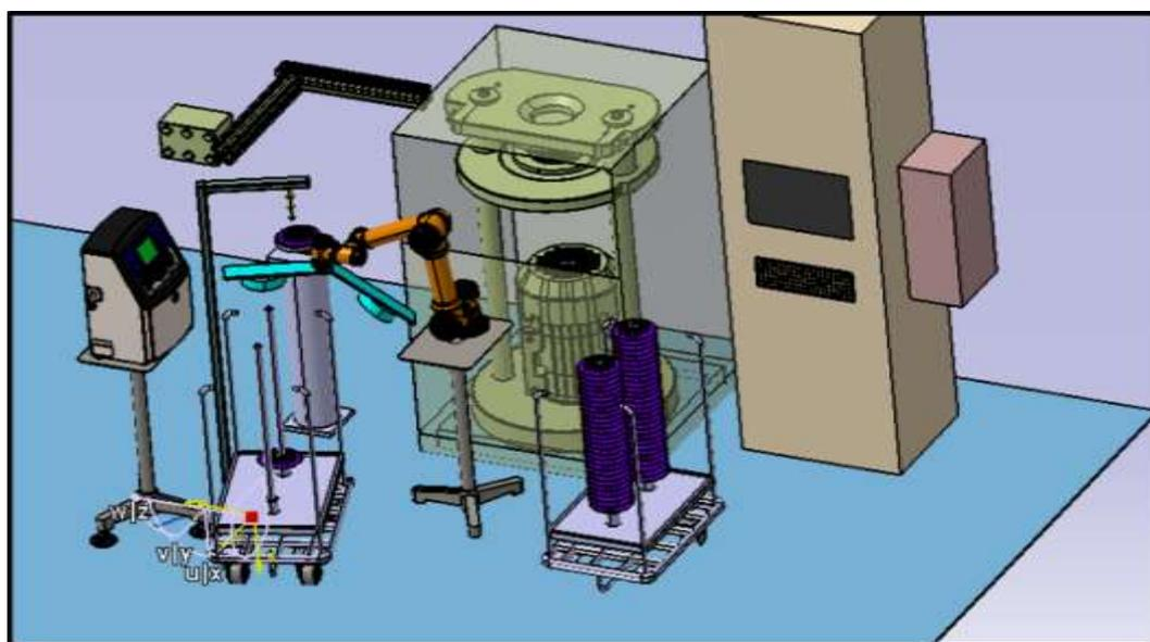
Figure 1 AUBO15 Robot with Electromagnetic Gripper in Clutch Diaphragm testing Process in DELMIA Software
