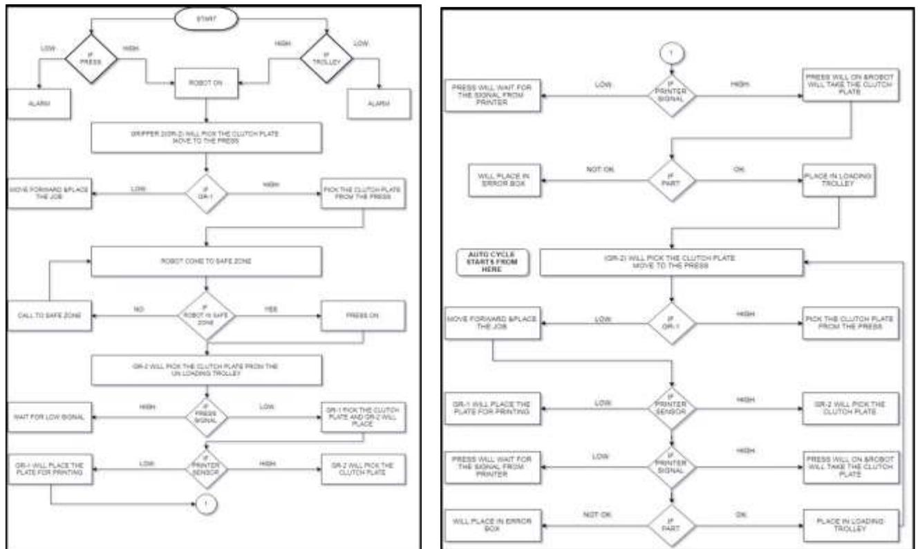
Figure.5 Flowchart for pick and place operation in clutch diaphragm spring testing robot.
