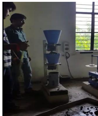
Compaction factor test apparatus
