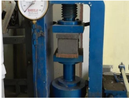
Testing of specimen at 7 days curing
