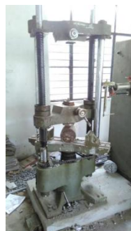
Split tensile strength testing at 14 days curing
