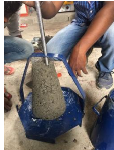
Slump cone test
