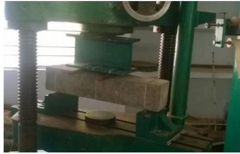
Testing Square prism for flexural strength
