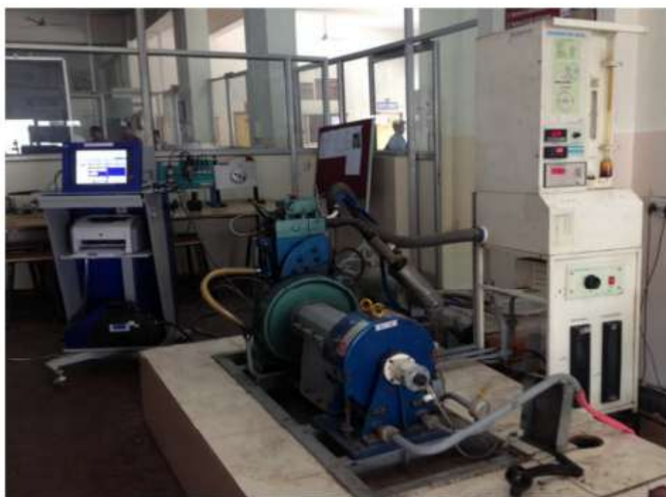
Figure 1 Experimental Setup with engine and analyzer
