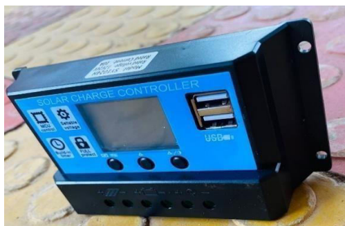
Fig 9 Solar charge controller
