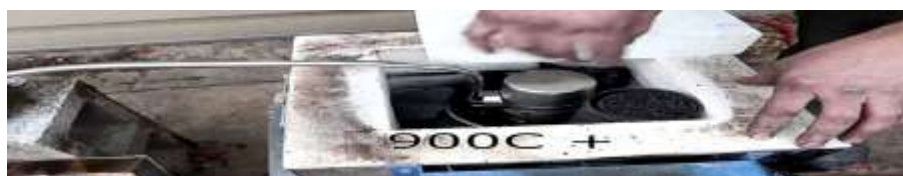
Fig 1:- Setup of Furnace to make Activated Carbon
