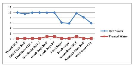
Graph 2: Comparison Turbidity between Raw Water and Treated Water
