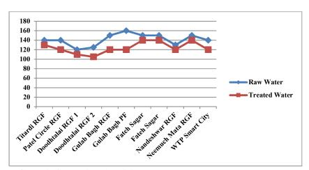
Graph 3: Comparison Alkalinity between Raw Water and Treated Water
