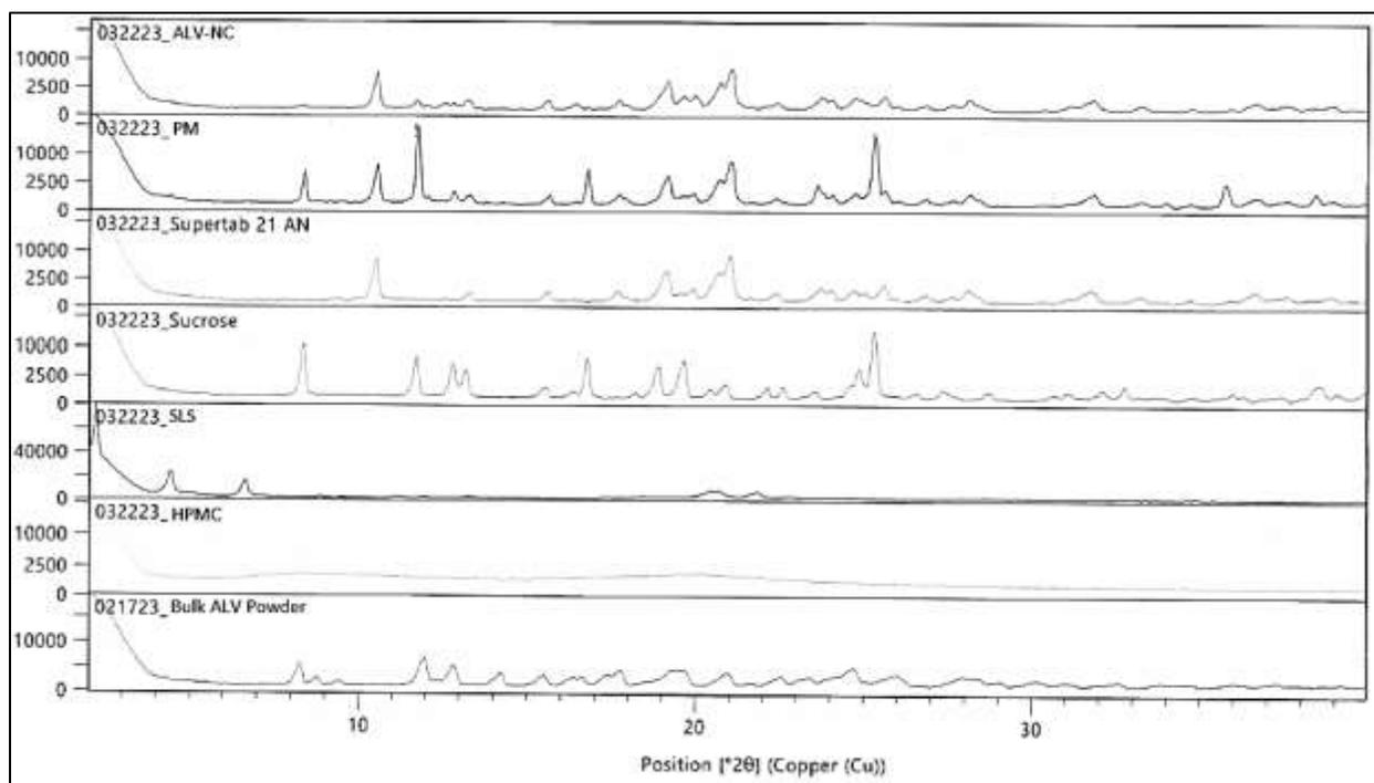
**Figure 5.** PXRD patterns of Bulk ALV powder, HPMC, SLS, Sucrose, SuperTab 21 AN, PM, and ALV-NC
