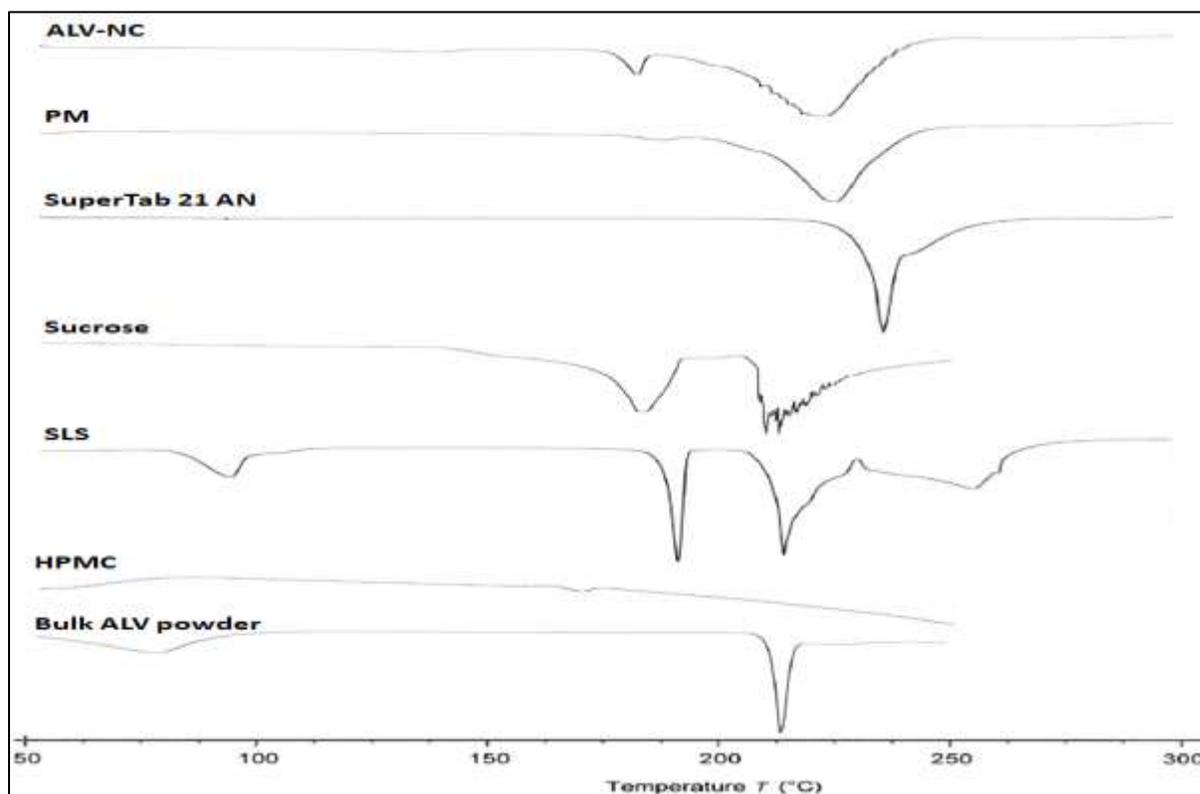
**Figure 4.** DSC images of bulk ALV powder, HPMC, SLS, Sucrose, SuperTab 21 AN, PM, and ALV-NC.
