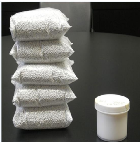
Fig 4: Both the 5 pounds of pellet concentrates and the 1/2 pound jar of liquid color will color 100 pounds of resin equally. [5]
