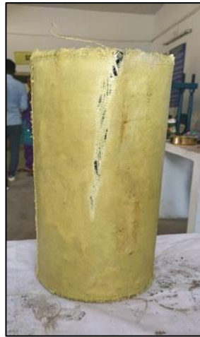
Fig.12 Failure mode of CC+2L Cylinder specimen
