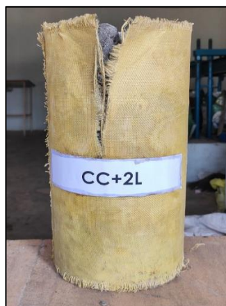
Fig.8 Failure mode of CC+2L Cylinder specimen
