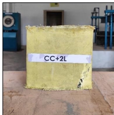
Fig.6 Failure mode of CC+2L Cube specimen
