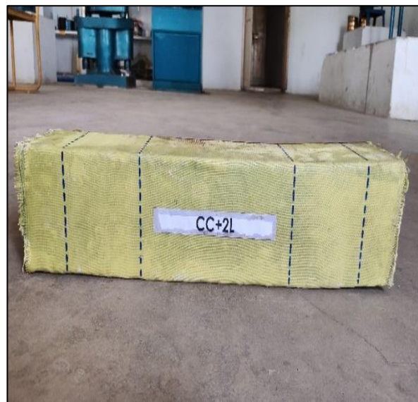
Fig.10 Failure mode of CC+2L prism specimen
