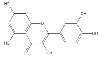
Figure 13, Chemical Structure of Quercetin
