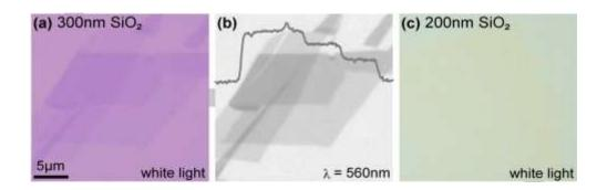
Fig 4: Microscopic image of graphene flake (a) on 300 nm SiO<sub>2</sub> (with white light), (b) green light and (c) on 200 nm SiO<sub>2</sub> (with white light). [16].
