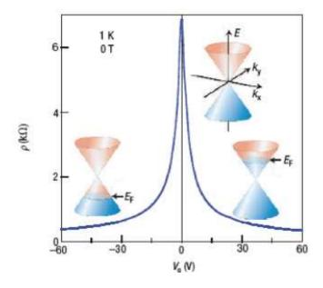
Fig 2: Figure showing ambipolar nature of single-layer graphene. Fig also depicts variations in the position of the EF of the Fermi energy with applying positive or negative gate voltage Vg [11].
