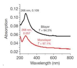
Fig 3: Absorption spectra of single layer and bilayer graphene in UV-Vis region showing absorption peak at 268 nm. The transmittance percentages are also shown measured at 550 nm (Fig adapted from paper [15]).
