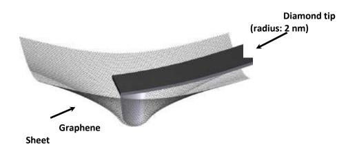
Fig. 6: An illustration of mechanical strength of graphene [21]
