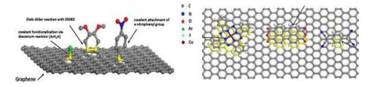
Fig 5: Illustration showing difference between (a) covalent and (b) non-covalent functionalization of graphene [18]
