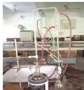
Fig 2. Extraction of essential oil from Matricaria chamomilla flower by using Clevenger apparatus
