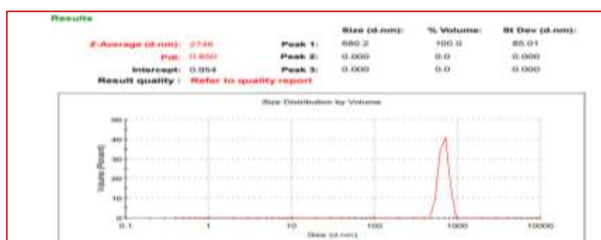
Fig. 3. Particle size distribution report graph of silver nanoparticles prepared by Alstonia scholaris Linn aqueous floral extract.
