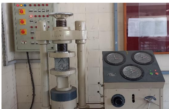
Fig. 5 Compressive Strength Testing Machine
