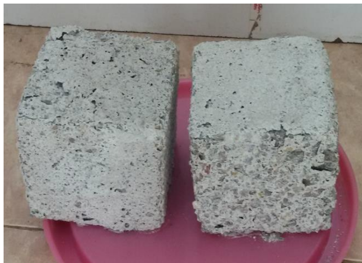
Fig. 14 Concrete sample exposed to acid ( \text{H}_2\text{SO}_4 ) attack
