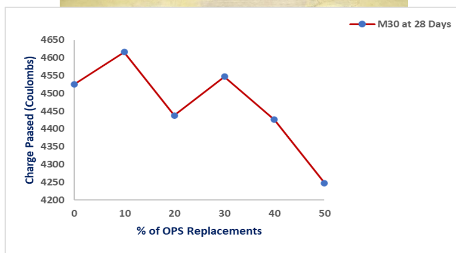
Fig. 13 Graph showing in charge passed for M30 grade OPS concrete at 28 Days
