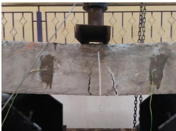
Fig. 9 Flexural crack occurrence in prism specimen
