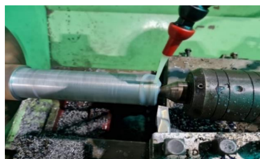
Fig.2: Experimental Setup-Mild Steel being turned with HSS tool bit and flood cooling.
