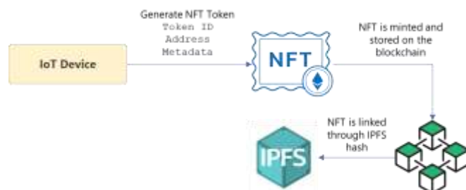
Fig. 4. The process of creating an NFT token for an IoT device
