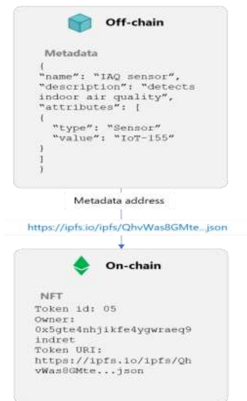
Fig. 5. ERC-721 tokens store NFT metadata on decentralized storage and token ID/metadata URI on-chain
