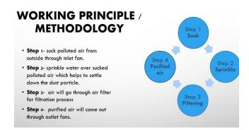
The air purifier further includes a plurality of exhaust fans to blow clean air out of the air purifier.
