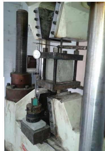
Figure 3 Test setup for pull out strength test
