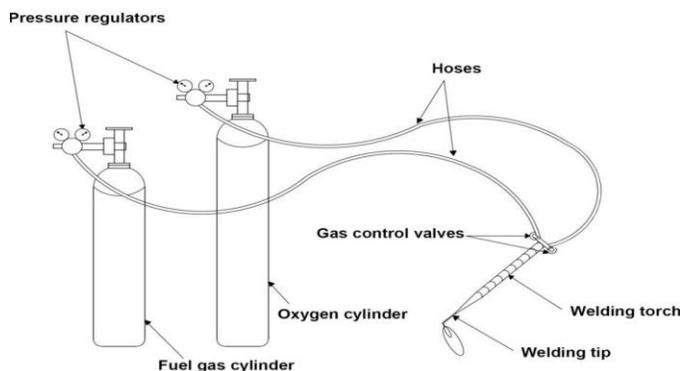
Fig. 3. Gas welding system (Source: Samir Hajili 2017)
