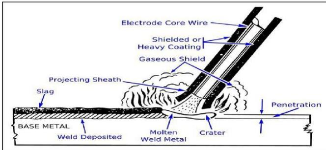
Fig. 4. Shielded metal arc welding process (Source: Hitesh Arora et al. 2019)
