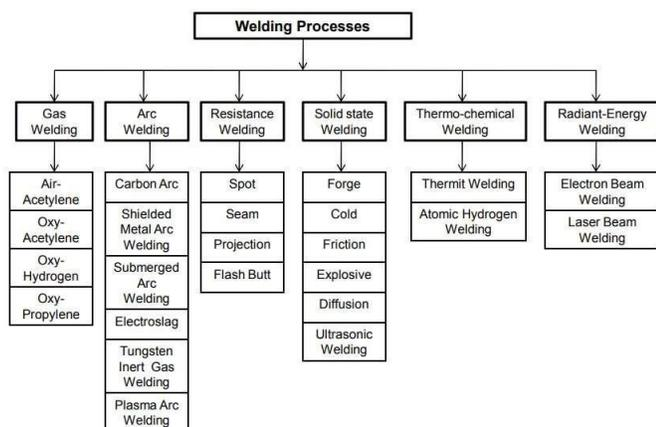
Fig. 2. Classification of welding process (Source: Welding Handbook: Volume Two, American Welding Society 1978)
