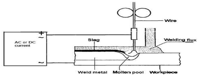
Fig. 5. Submerged arc welding process (Source: KlasWeman 2003)
