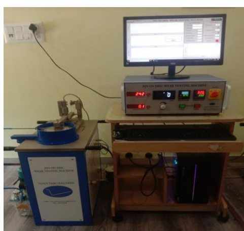
Figure 3.6. Wear Testing Apparatus
