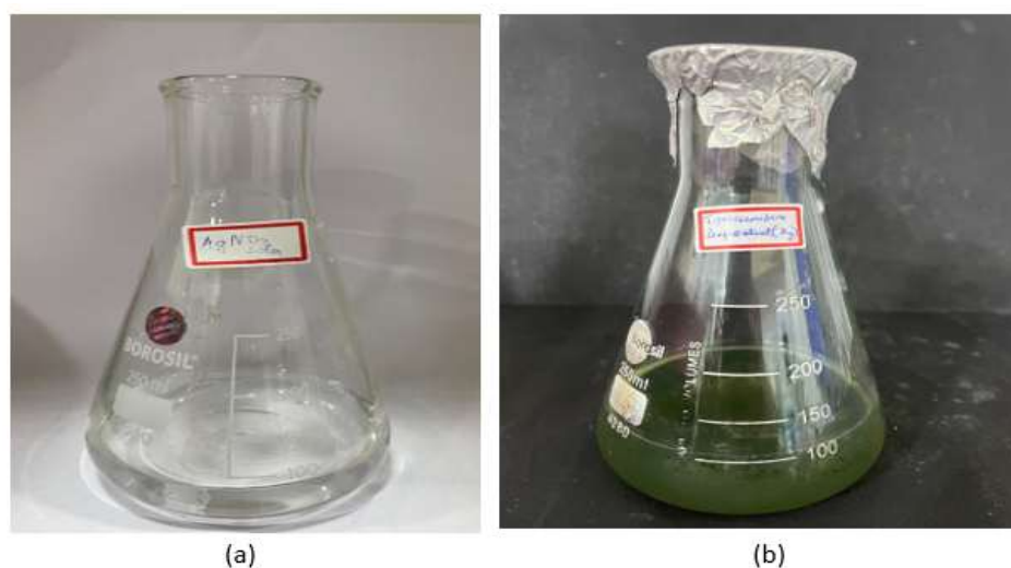
Figure 2: Synthesis of silver nanoparticles from T. procumbens leaves extract (a) \text{AgNO}_3 solution (b) T. procumbens leaves extract dissolved in \text{AgNO}_3 solution
