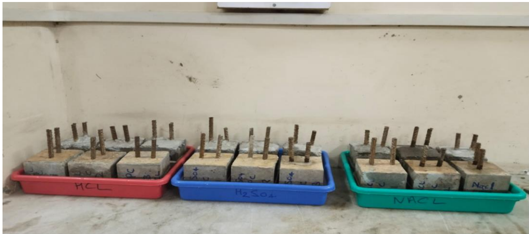
Cubes Partially immersed in 3% HCL, H 2 SO 4 , NACL for 56 days
