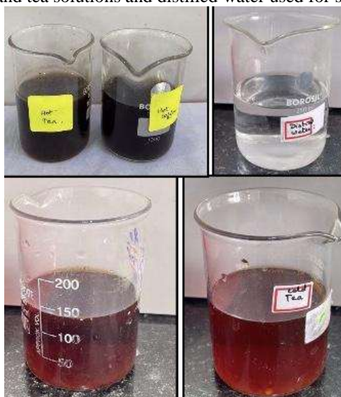
Figure 2: Prepared coffee and tea solutions and distilled water used for storing composite specimens
