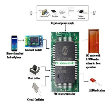
The project "Door Access using Voice Recognition" was designed a voice command-based door controlling system which is operated wirelessly through smart phone via Bluetooth. The receiver receives the signal from the phone and sends to the Microcontroller which send commands to open or close the door. A phone is used as a remote for controlling the door to be locked or unlocked.
