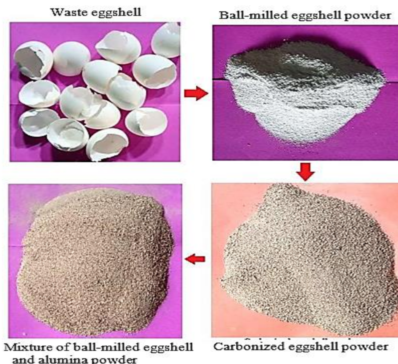
Figure 3: Eggshell and alumina converted into the carbonized form
