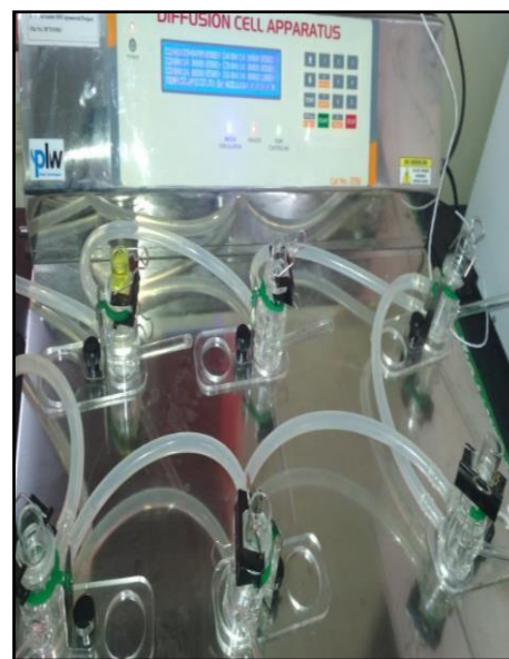
Figure 16: Permeation study through Franz diffusion cell
