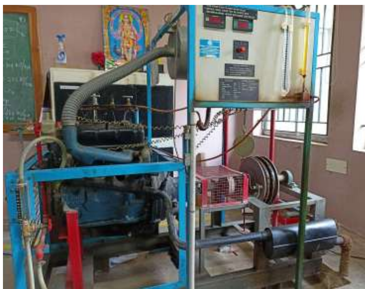
Fig. 2. Multi cylinder engine test bed of Hindustan motors Ambassador vehicle
