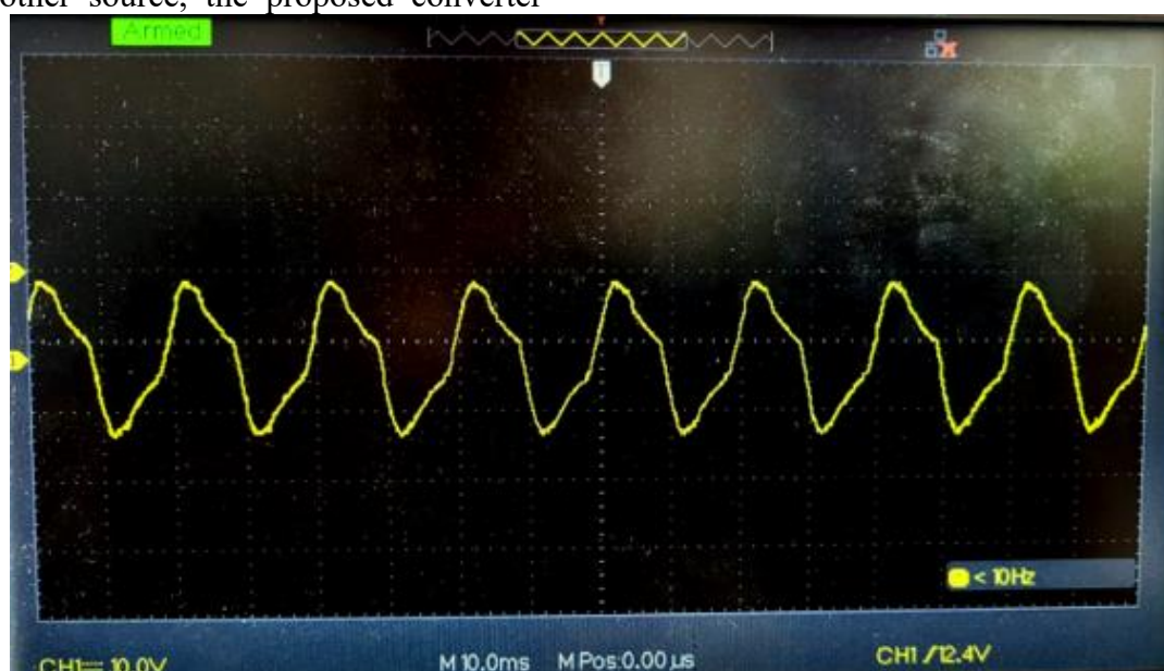
Fig.7- Output Waveform of hardware (Across the inductor L_1 )
