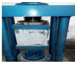
Compression testing machine testing sample specimen
