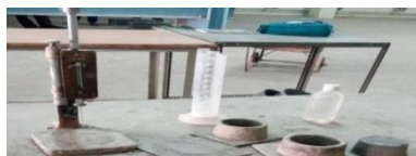
Fig 4. 2 : vicat apparatus Initial setting time of cement test results
