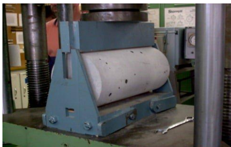
Split tensile machine test specimen sample
