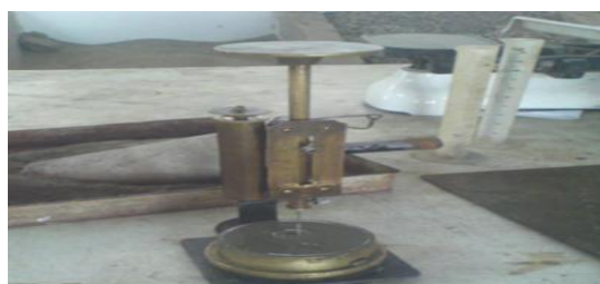
Fig 4. 1 : Normal consistency of cement
