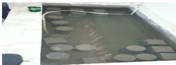
Curing of cubes and cylinders.
