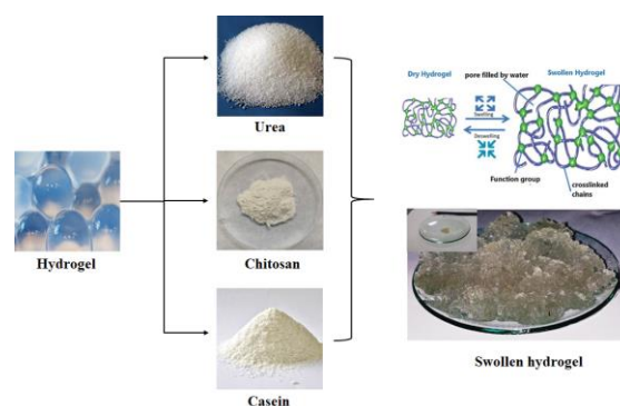
Figure 3: Composition and manufacturing process of hydrogels
