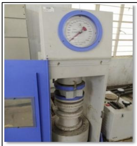
Fig. 4 Compression test on paver block specimen
