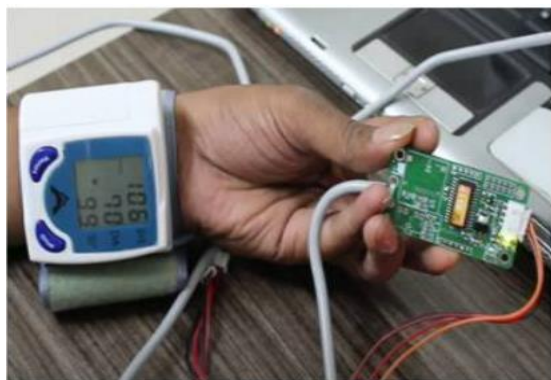
Fig. 4 : Patient's data collection using Blood pressure Sensor
