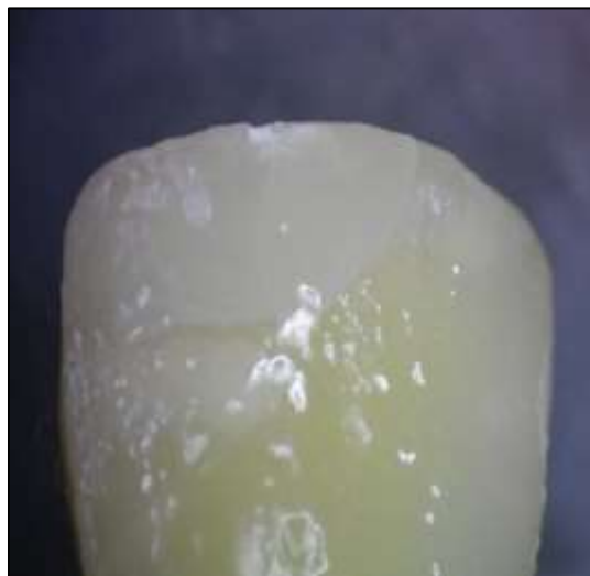
Figure (2): Edge chipping under stereo microscope
