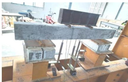
Figure 7 displays the 4 point load test configuration for the RC beam specimen
