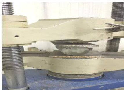
Fig. 4 Test setup of Split Tensile Strength Test
