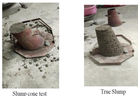
Fig.2 Slump Cone Test
