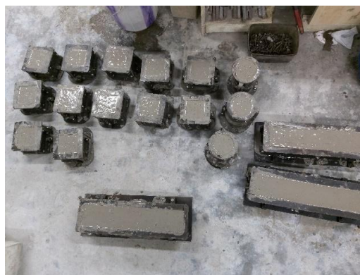
Fig.1 Casting of Specimen
