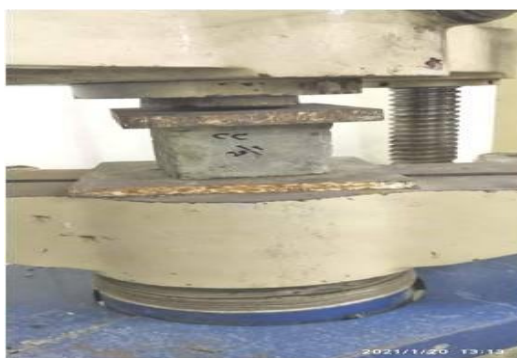
Fig. 3 Testing Setup of Compressive Test
