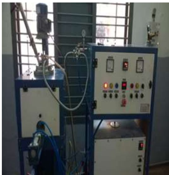
Figure 5 Induction furnace used for the preparation of MMCs
