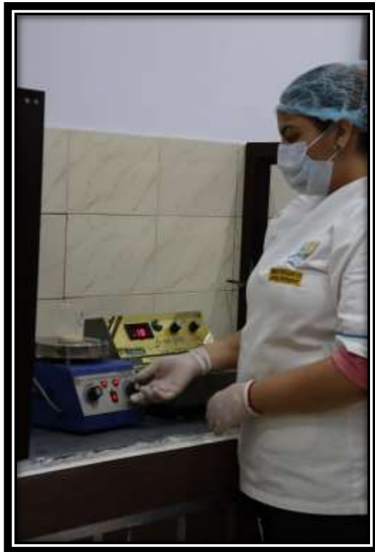
Figure: 1 Mixture Preparation Magnetic Stirrer
