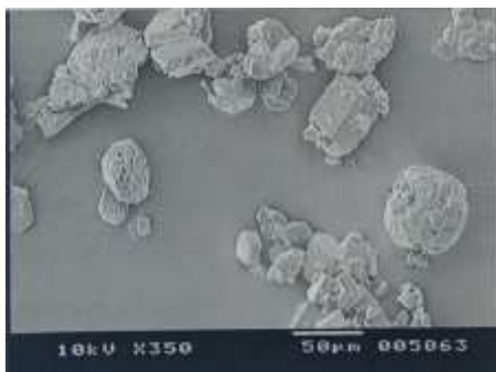
Fig: No:5 Scanning Electron Microscopy of Spherical Agglomerates at 800 rpm
