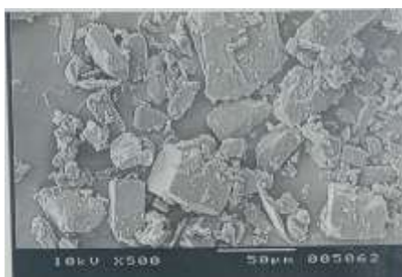
Fig: No:3 Scanning Electron Microscopy of Pure Gliclazide
