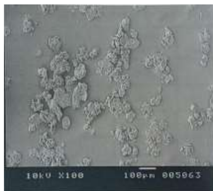
Fig: No:6 Scanning Electron Microscopy of Spherical Agglomerates at 100 rpm
