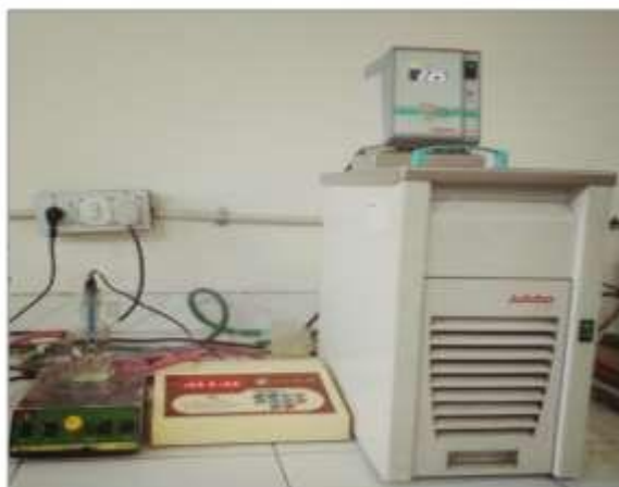
Digital conductivity meter (Model: Systronics-306) connected with a temperature bath used for conductivity measurements.
