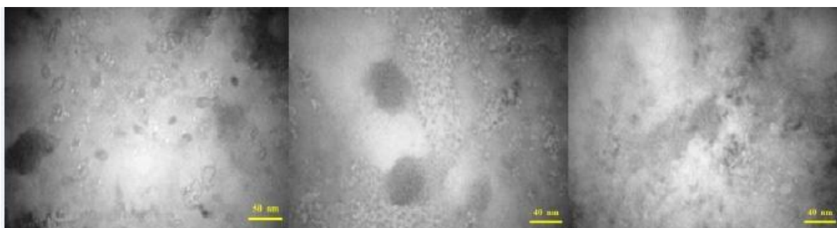
Figure 4. TEM images of the CdS quantum dots
