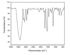
Fig 13:FTIR spectra of porous slab with microalgae
