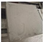
Fig 7: Non-porous geopolymer slab
