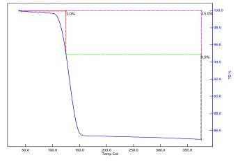
Fig 14.TGA curves of the specimen
