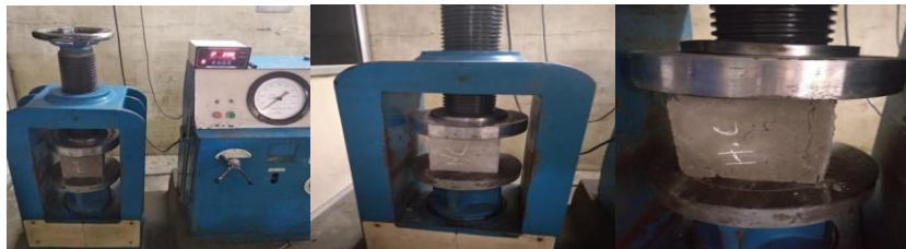
FIGURE:1 Testing of Cube for compressive strength
